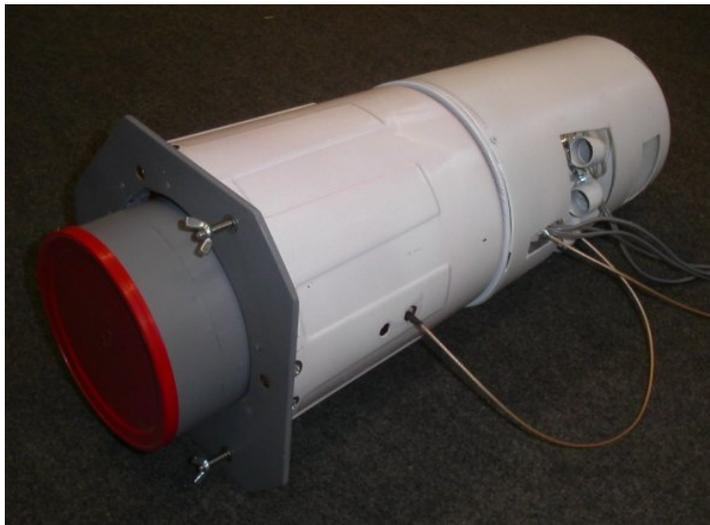
Figure 6 Complete Head Amplifiers and cylindrical feed assembly
